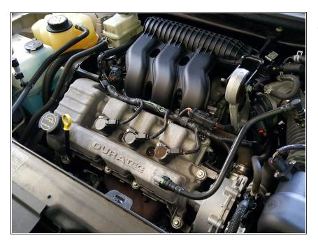
Now that the refrigerant has been removed professionally, it's your turn to go to work. Pop the hood of a 2005-2007 Ford Freestyle, Ford 500, or Mercury Montego and you're looking at a 3.0L V6 DOHC 24V DURATEC engine. This was the one and only engine option for these vehicles.
