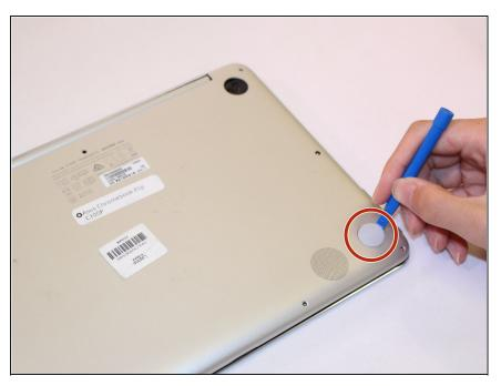
Use the plastic opening tool to remove the four bottom rubber feet.
