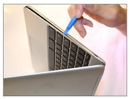
• Use the plastic opening tool to pry up the palm rest assembly.
