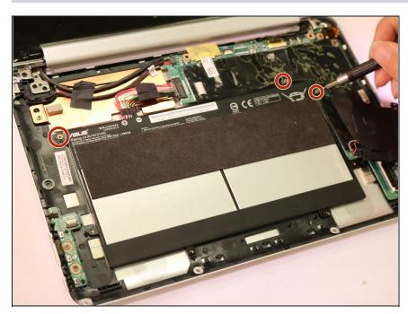
• Unscrew the three Battery Screws by using a screwdriver with a J00 tip.
