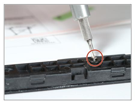
Using the "PH000 driver" to remove the 6 three-millimeter screws around the battery casing. All 6 screws are circled in red in the image seen in step 2.
