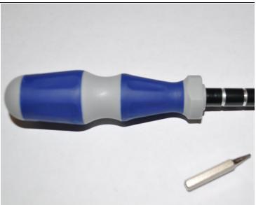
Using a T-5 Torx screwdriver, remove all four screws at the back of the device by turning them counterclockwise. A sample screwdriver is located here.
