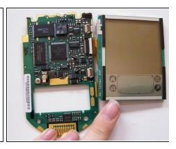
Remove the back and front cover from the interior parts of the device.
