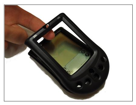
• Unclip the tab at the top of the device, to remove the face plate.
