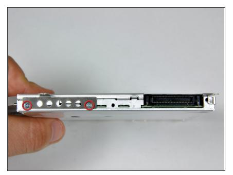
Remove the two Phillips screws securing the mounting bracket to the rear of the optical drive.
