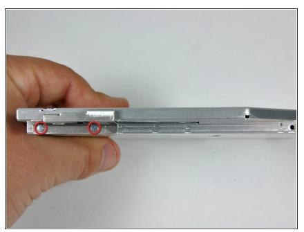
Rotate the drive and remove the two Phillips screws securing the mounting bracket to the right side of the optical drive.
