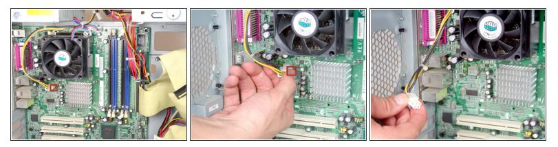
Remove the 4 pin ATX power connector from the motherboard by pressing down the holding latch and pulling out towards the side of the device.
