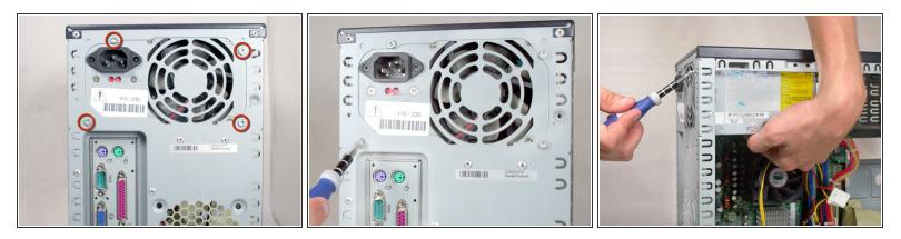
Remove the 4 Torx T15 screws from the rear of the power supply
