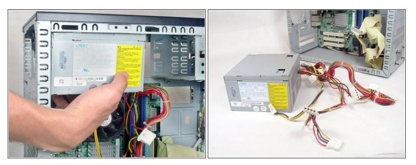
• Slide the power supply towards the front of the device
