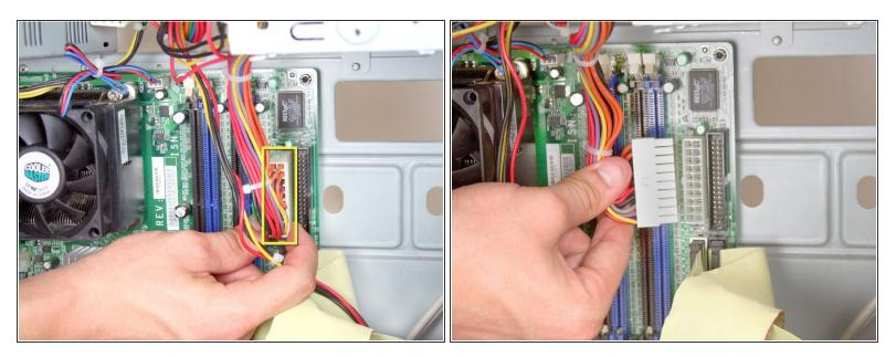
• Remove the 20 pin ATX power connector from the motherboard by pressing down the holding latch and pulling out towards the side of the device.
