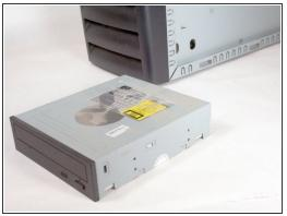
Remove the optical drive by sliding it out the front of the device.
