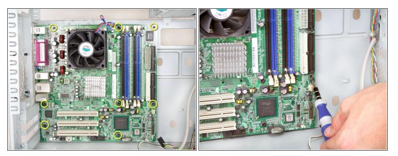
Remove the 8 Torx T15 screws from the motherboard.
