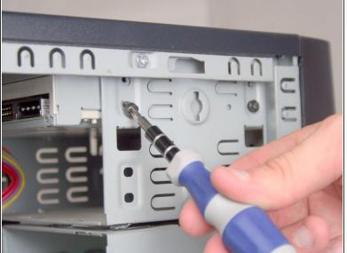
• Remove the 2 Torx T15 screws holding the optical drive in place.
