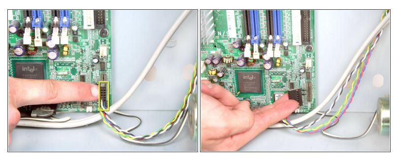
Remove the 16 pin connector from the motherboard by pulling it out towards the side of the device.
