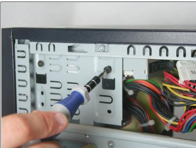
Remove the other 2 Torx T15 screws holding the other side of the drive in place.
