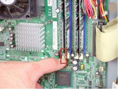
Release the lower portion of the RAM by pushing down on the bottom tab.
