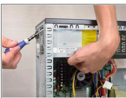
Remove the 4 Torx T15 screws from the rear of the power supply
