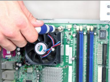
Unscrew the 4 Torx T15 screws holding the CPU Cooler in place.
