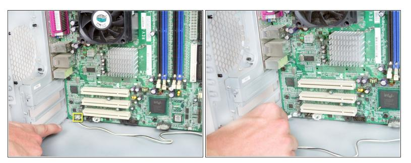
Remove the 2 prong speaker connector by pulling out towards the side of the device.
