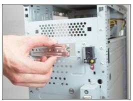
Remove the external drive faceplate by removing the two Torx T15 screws.
