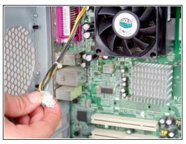
Remove the 4 pin ATX power connector from the motherboard by pressing down the holding latch and pulling out towards the side of the device.
