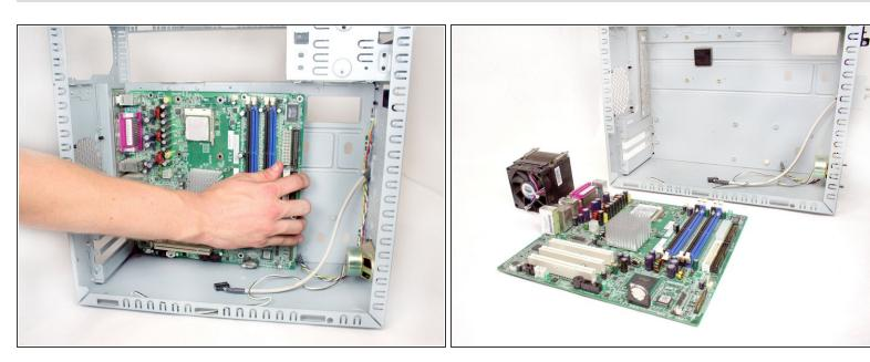
Remove the motherboard by pushing it forwards and removing it from the case.
