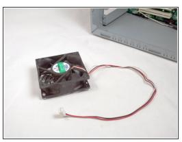
Remove the fan from the case by pulling it towards the front of the device.
