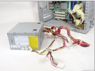
Slide the power supply towards the front of the device
