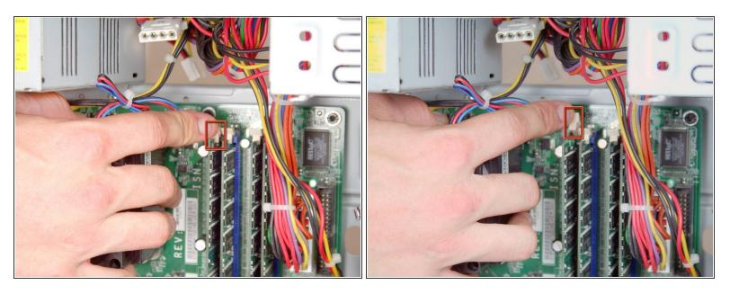
Release the upper portion of the RAM by pushing down on the upper tab.
