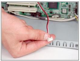
Remove the 3 prong power connector from the motherboard by pulling it outwards toward the side of the device.
