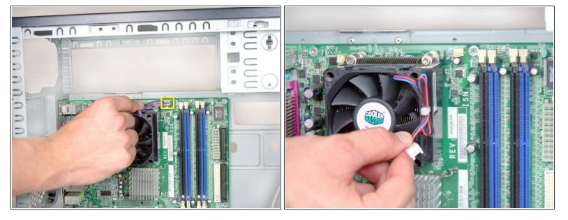
Remove the 3 pin power connector by pulling it out towards the side of the device.
