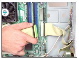
Remove any IDE cables from the motherboard by pulling them out towards the side of the device.
