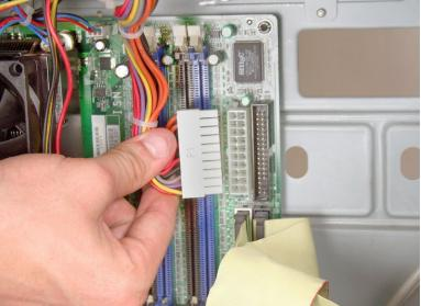
Remove the 20 pin ATX power connector from the motherboard by pressing down the holding latch and pulling out towards the side of the device.
