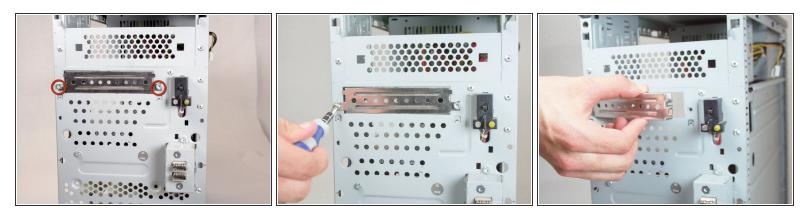
Remove the external drive faceplate by removing the two Torx T15 screws.
