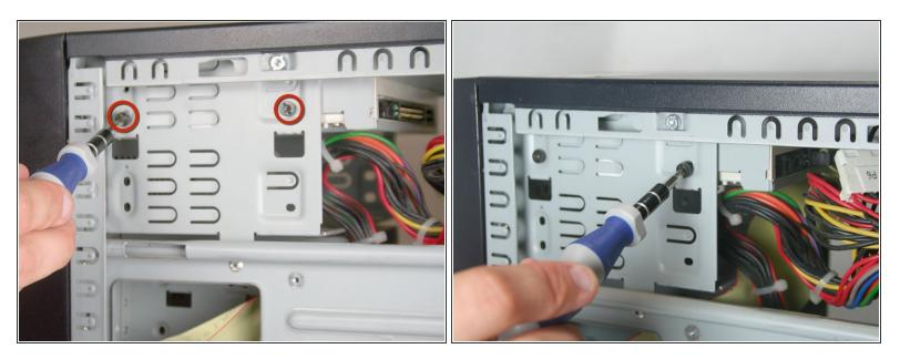
• Remove the other 2 Torx T15 screws holding the other side of the drive in place.
