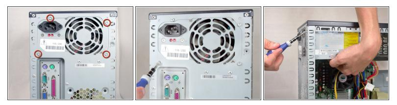
Remove the 4 Torx T15 screws from the rear of the power supply
