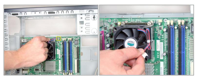
• Remove the 3 pin power connector by pulling it out towards the side of the device.
