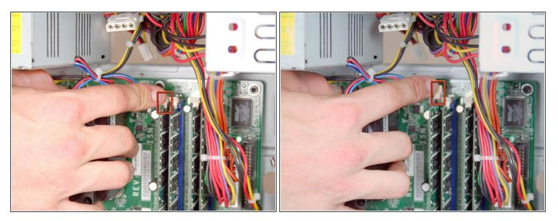
• Release the upper portion of the RAM by pushing down on the upper tab.
