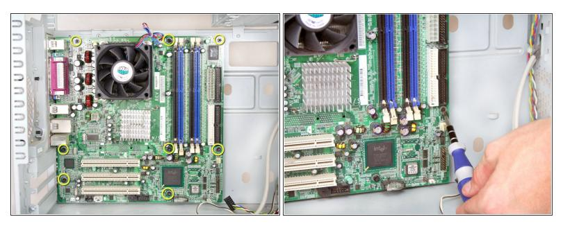
• Remove the 8 Torx T15 screws from the motherboard.
