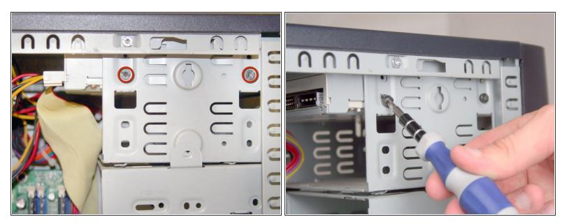
• Remove the 2 Torx T15 screws holding the optical drive in place.
