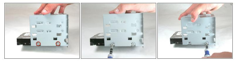
• Remove the two Torx T15 screws holding this side of the hard drive in place.
