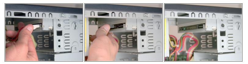
Remove the IDE data cable and the power cable from the optical drive by pulling away from the drive.
