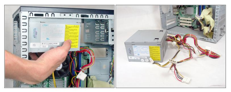
• Slide the power supply towards the front of the device
