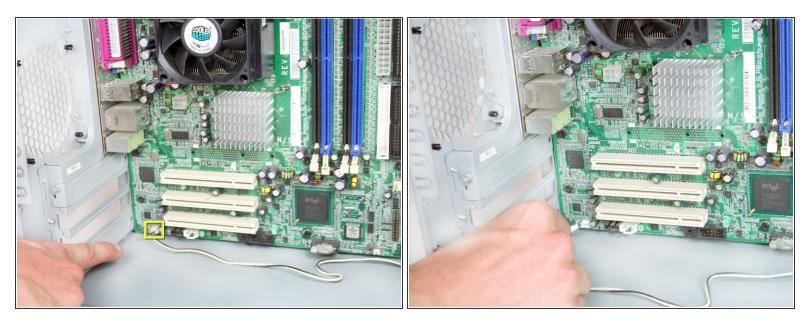
• Remove the 2 prong speaker connector by pulling out towards the side of the device.
