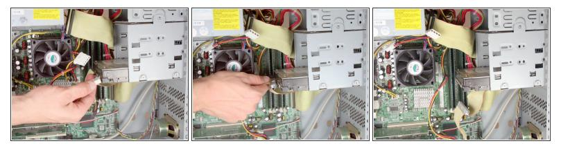
• Remove the IDE data and power cables from the hard drive.
