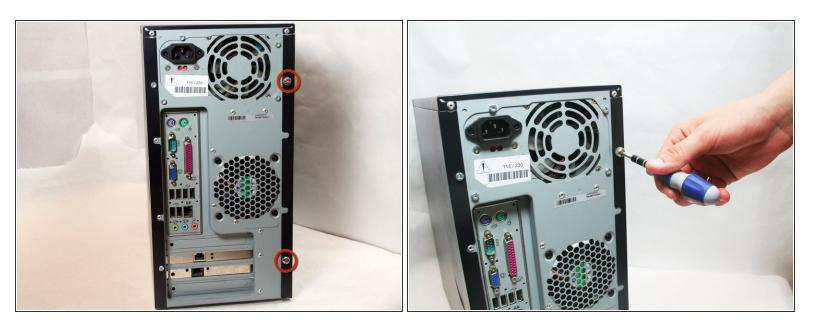
Remove the two Phillips #2 screws that secure the case door to the device.
