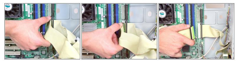
• Remove any IDE cables from the motherboard by pulling them out towards the side of the device.
