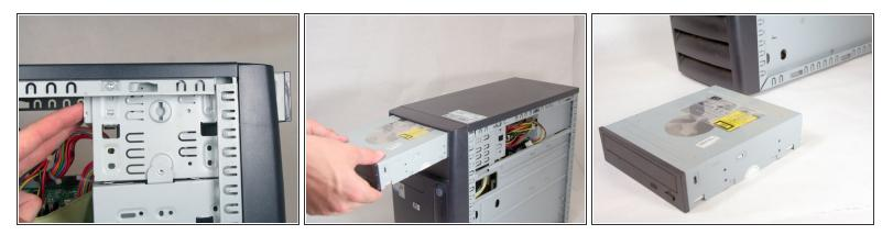
• Remove the optical drive by sliding it out the front of the device.
