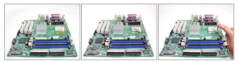
• Lift up the bar that secures the processor to the motherboard
