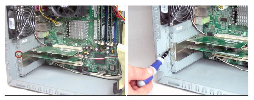
Remove the Torx T15 screwdriver holding the PCI card in place.
