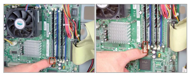
• Release the lower portion of the RAM by pushing down on the bottom tab.
