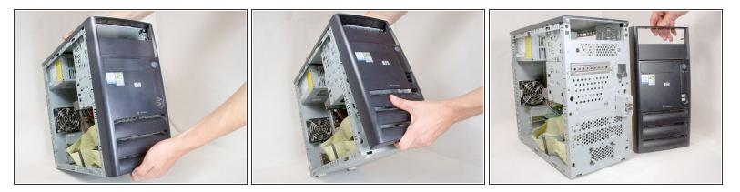
• Remove the front bezel by pulling upwards and out from below the lowest air vent.
