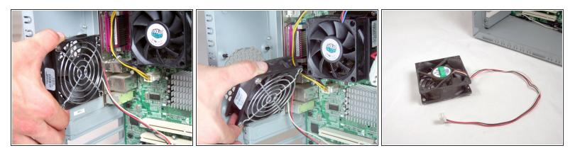
• Remove the fan from the case by pulling it towards the front of the device.
