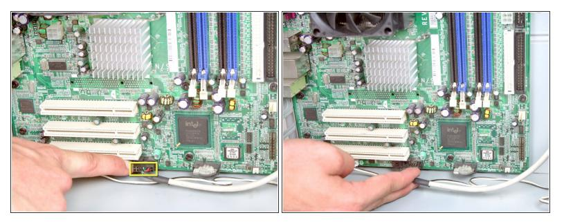
• Remove the 14 pin USB connector by pulling it out towards the side of the device.
