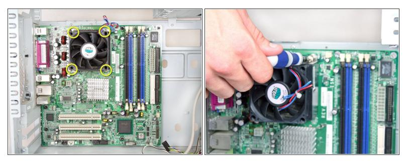
• Unscrew the 4 Torx T15 screws holding the CPU Cooler in place.
