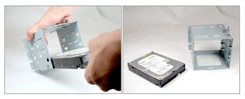
• Remove the hard drive from the hard drive cage by pulling it outward from the cage.
