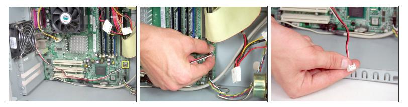
Remove the 3 prong power connector from the motherboard by pulling it outwards toward the side of the device.
