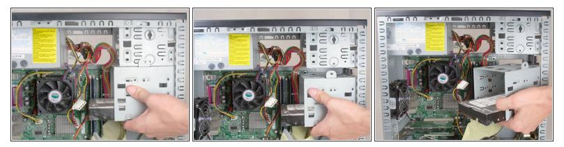
• Fully remove the hard drive cage by sliding it towards the back of the device and pulling down.
