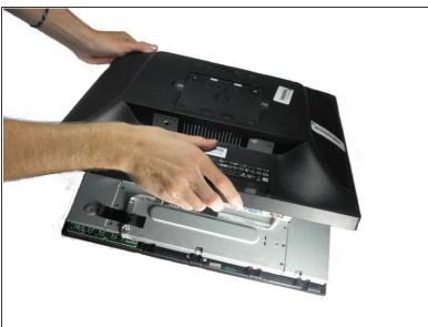
When finished prying, the plastic will partially fall away from the rest of the monitor.
