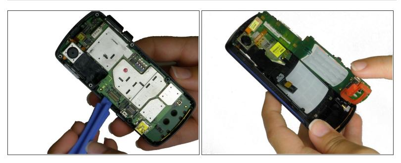
Use a plastic opening tool to gently pry the motherboard up until you can tilt it with your fingers.
