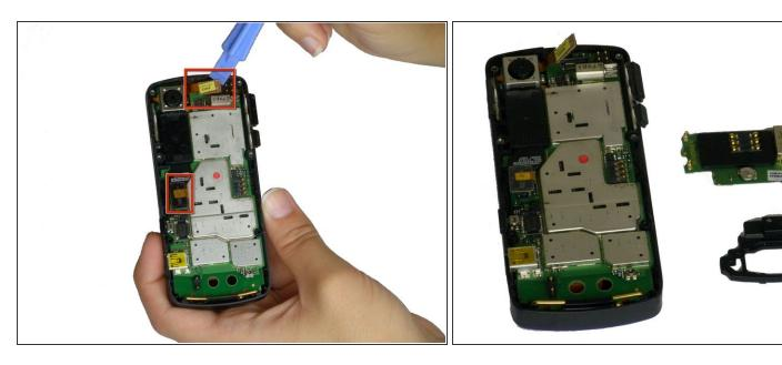
Use a plastic opening tool to pry the two ribbon cable connectors, unclipping them from their sockets on the motherboard.
