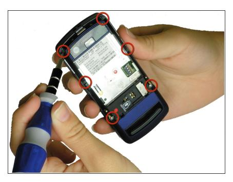
Use a T4 screwdriver to unscrew all six of the .216 inch screws that attach the housing to the case.
