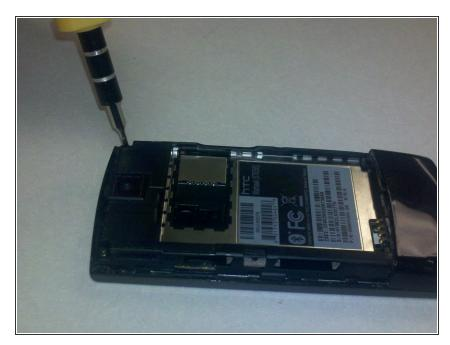
• Unscrew the two screws on the back of the phone with a T5 screwdriver
