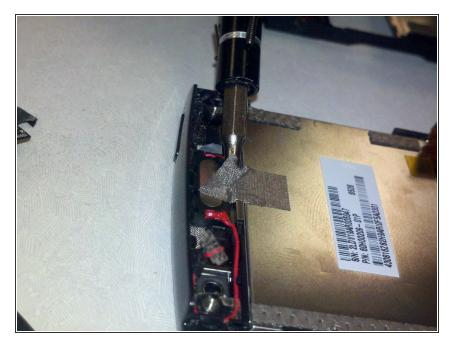
Next take the SL#2.5 screwdriver and pry the grey fabric sticker off on the LCD side of the phone
