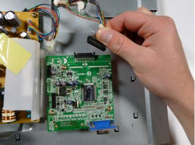
Remove the display cable located at the top of the motherboard by pulling it out towards the top of the monitor.
