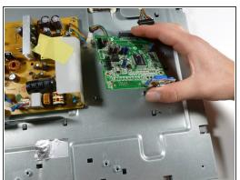
Remove the three 7.7 mm Phillips #2 screws from the motherboard, and take out the motherboard by lifting it up.
