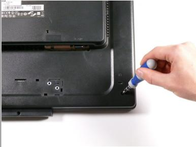
Remove the five 9.5 mm Phillips #2 screws located around the perimeter of the monitor.
