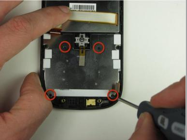
Remove the four 1.9 mm Phillips #00 screws.
