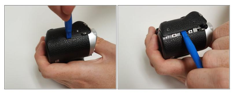
Use the plastic opening tool in a downward motion around each side of the camera to pry the casing open.
