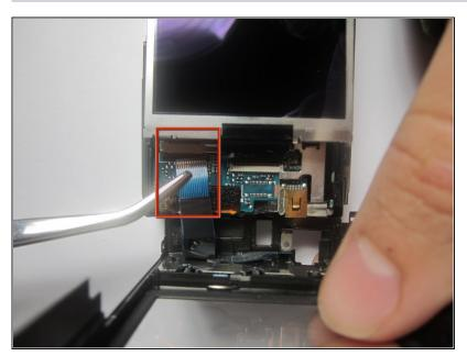
Use the <u>tweezers</u> to disconnect the ribbon from the circuit board.
