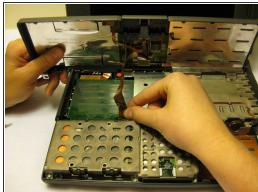
• Remove the front plastic panel of the laptop by carefully lifting it up.
