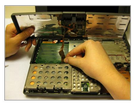
Remove the orange stripped ribbon that connects the trackpad to the rest of the laptop by carefully pulling up.
