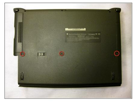
With the laptop upside down and with the battery removed, use a Torx #9 screw driver to remove the three .84 in. screws shown.
