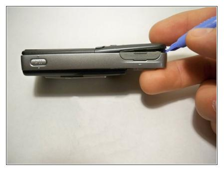
• Gently pry open the front casing by working an opening tool along the entire seam.
