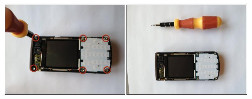
• Use the T6 Torx screwdriver to remove the six 15 mm Torx screws.
