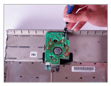
Use a T8 torx screwdriver to remove the six, 6.8mm long screws from the top of the green circuit board.
