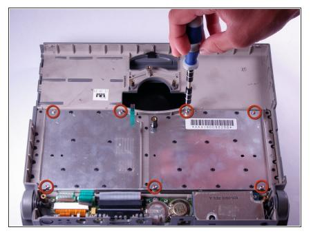
Use a T8 torx screwdriver to remove the seven, 6.8mm long screws from the metallic panel.
