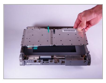
Remove the keyboard by lifting it vertically away from the main body of the computer.
