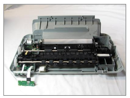
Turn the printer back down so that it is sitting on the bottom panel and rotate the printer 180 degrees.
