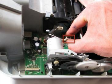
Disconnect the page sensor from the logic board by pulling straight up on the connector.
