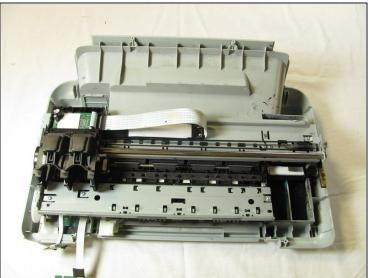
• Gently push the ink cartridge carriage to the left side of the printer.
