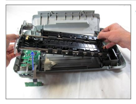
Lift the feed roller assembly straight up to remove it.
