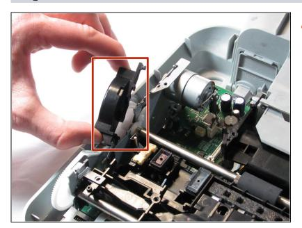
Remove the plastic gear cover by pulling it away from the printer body and lifting it up.
