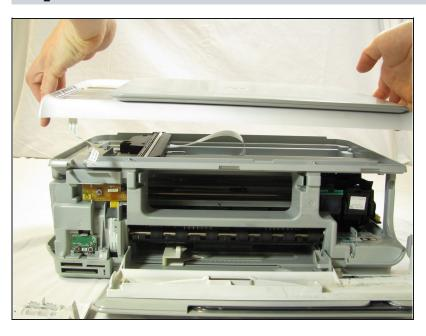
Carefully lift the top panel of the printer away from the printer body.
