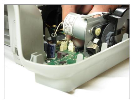
Carefully remove the connector holding the drive motor wires to the main circuit board.
