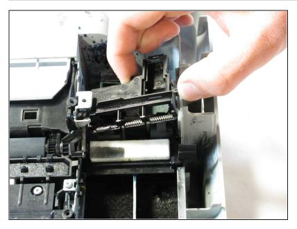
Remove the pad holder by lifting it straight up.
