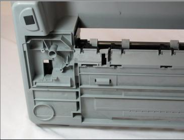
• Remove the black plastic cross member from the bottom of the printer.
