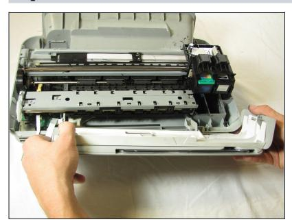
Remove the printer door and paper tray by putting them in the closed position and not laying flat then rotating them upwards lift the left side up.
