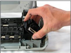
• Remove the printer head cleaner by lifting the front of the printer head cleaner above the track and slide it forward.
