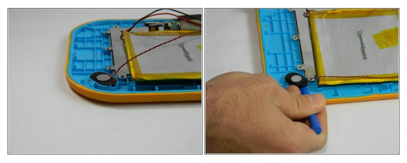
• Using the plastic opening tool, gently pry the speaker out of its plastic housing.
