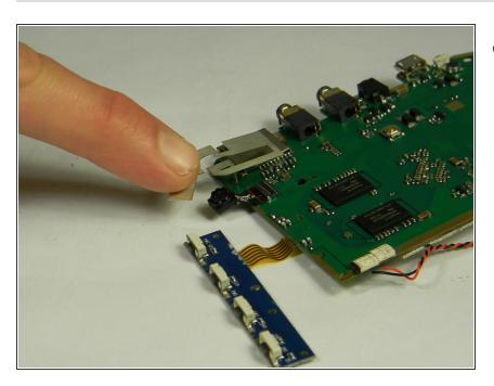
Gently slide out the ribbon wire connecting the camera to the motherboard.
