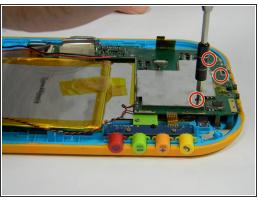
Unscrew the five 4 mm screws around the perimeter of the motherboard using the ph00 size phillips head screwdriver.
