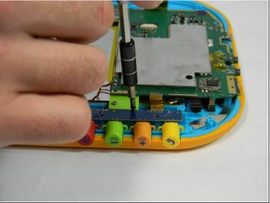
Remove the button board by unscrewing two more 4 mm screws and one 6.5 mm screw
