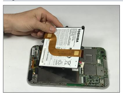
Battery will lift out of the device.
