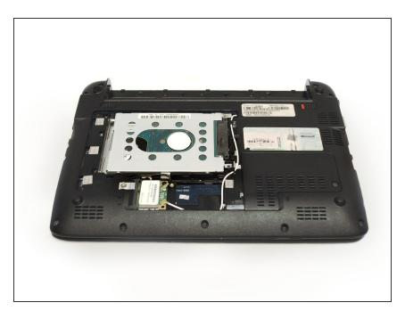
Locate the HDD after the back plate is removed. It will be the large rectangle that takes up most of the space.
