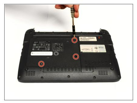
Use a #0 Phillips screwdriver to remove the three 6mm screws from the larger back plate.
