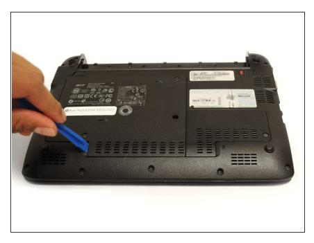
Use the plastic opening tool on the recessed notch at the bottom of the larger plate to gently lift the plate.
