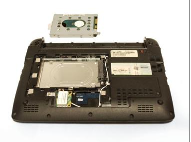
Grab the edges of the HDD, slightly rotate it, and gently pull it out.
