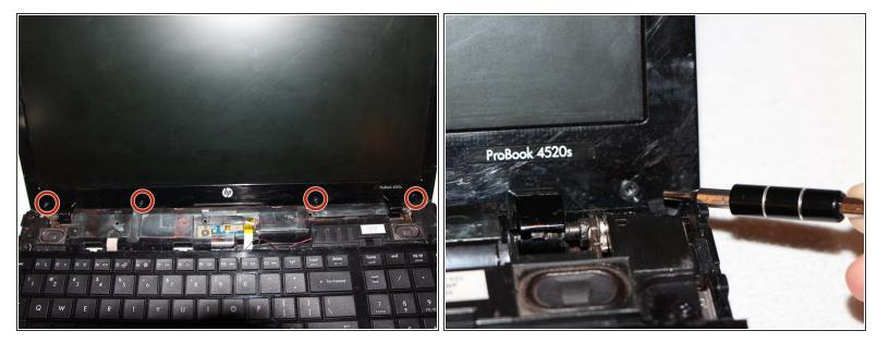
• Use a Torx (T9) head screwdriver to remove the four 5mm screws beneath the rubber caps.
