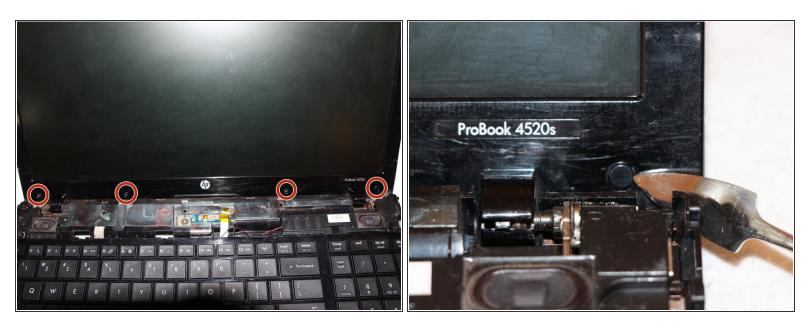
Use a metal spudger to remove four rubber caps at the bottom of the screen border.
