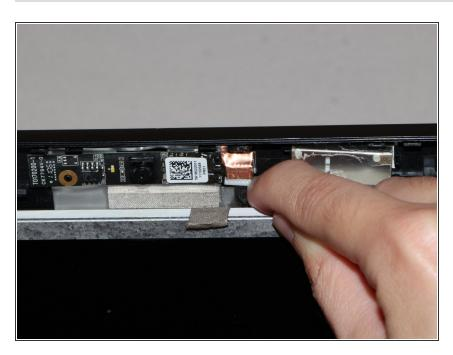
Above the screen is a bronze port with a cable connected to it.
