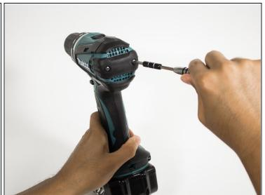
• Unscrew two 18mm screws from the back panel with the Phillips PH2 screwdriver.
