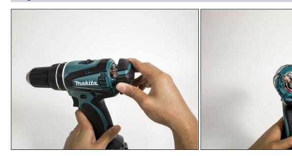
Apply slight pressure to the sides of the backplate and pull away from the drill.
