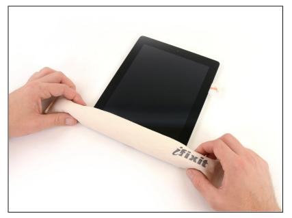
While you work on releasing the adhesive on the right side of the iPad, reheat the iOpener, and replace it on the bottom edge of the iPad.
