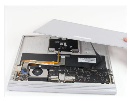
Lift the panel away with the ribbon cable still attached and set aside the panel so that you can work on other components.
