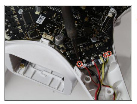
Desolder the red, yellow and black wires that connect the LED to the control board. Check out the link below for more information on desoldering. <u>Desoldering</u> <u>Information</u>
