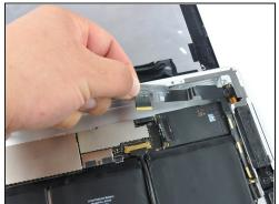
• Use the flat end of a plastic opening tool to flip up the retaining flap on the headphone jack and front-facing camera ribbon cable ZIF socket.
