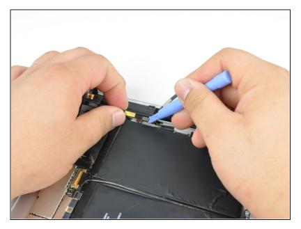
Use the edge of a plastic opening tool to disconnect the microphone cable connector.
