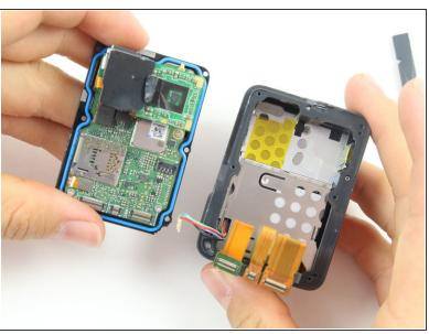
• Use the flat end of the spudger to pry the battery housing power cable straight up from its socket on the motherboard.
