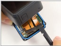
Use the flat end of a spudger to pry the three ribbon cables connected to the side of the motherboard.
