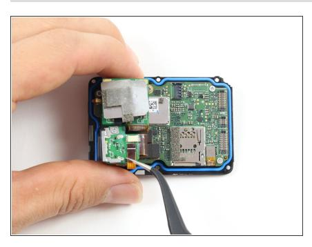
Use the tweezers to pull the ribbon cable connector out of its white socket on the charging assembly board.
