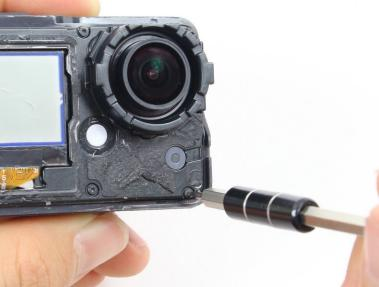
Remove the six T3 Torx screws.
