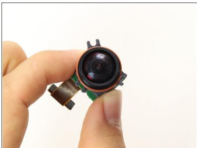
Pull the lens assembly straight out from the Midframe.
