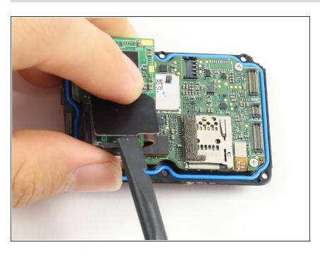
Use the flat end of the spudger to pry the black cover plate straight up from its socket on the motherboard.
