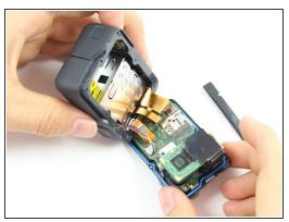
⚠ Be careful when pulling open the motherboard assembly as it is still connected to the back housing by four cables. The cables may break if stretched.
