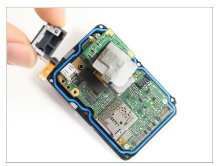
Remove the charging assembly housing by pulling it straight up off the motherboard.
