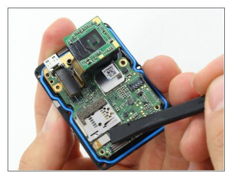
Use the flat end of the spudger to pry the LCD screen ribbon cable connector straight up from its socket on the motherboard.
