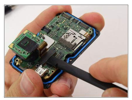
Use the flat end of the spudger to pry the lens assembly ribbon cable connector straight up from its socket on the motherboard.
