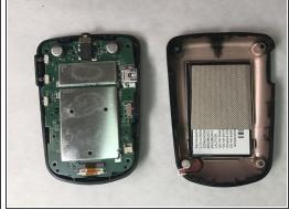
Use the blunt tweezers to unplug the battery cable from the PCB board. Grab the battery cable plug from the sides.
