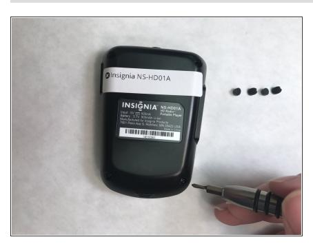
Remove the four 6.0 mm Phillips screws located below the rubber caps using the PH00 bit installed in the driver.
