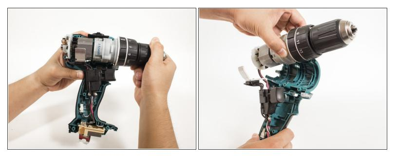
Grip the motor comfortably towards the front of the assembly, and pull it away from the outer casing.
