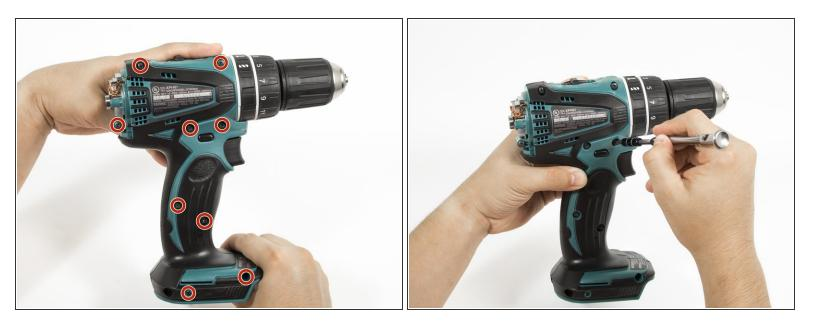
Unscrew the nine 18 mm screws from the outer casing using a Phillips PH2 screwdriver.
