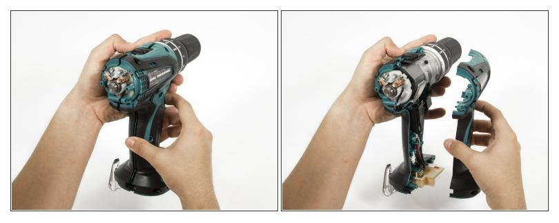
• Apply slight pressure to the sides of the outer casing and pull away from the drill.
