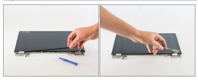
• Remove the LCD hinge cover by gently prying the pieces with a plastic spudger and lifting the hinge cover up and out.
