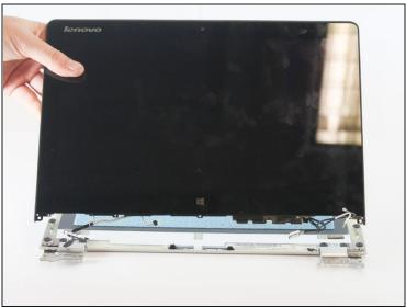
• Remove the LCD by carefully pulling away from the hinges and upwards.
