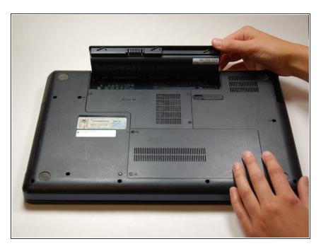
Remove the battery, carefully, from the compartment.
