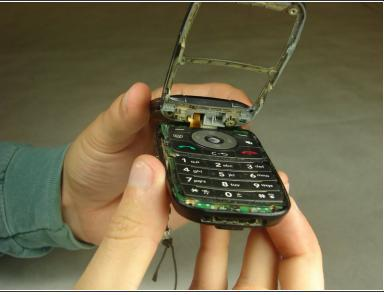
Once you have worked your way around the perimeter of the phone, you will have access to the components in the bottom half assembly. To reassemble your device, follow these instructions in reverse order.
