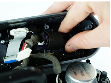
Remove the battery cover plate carefully then proceed to remove the battery.
