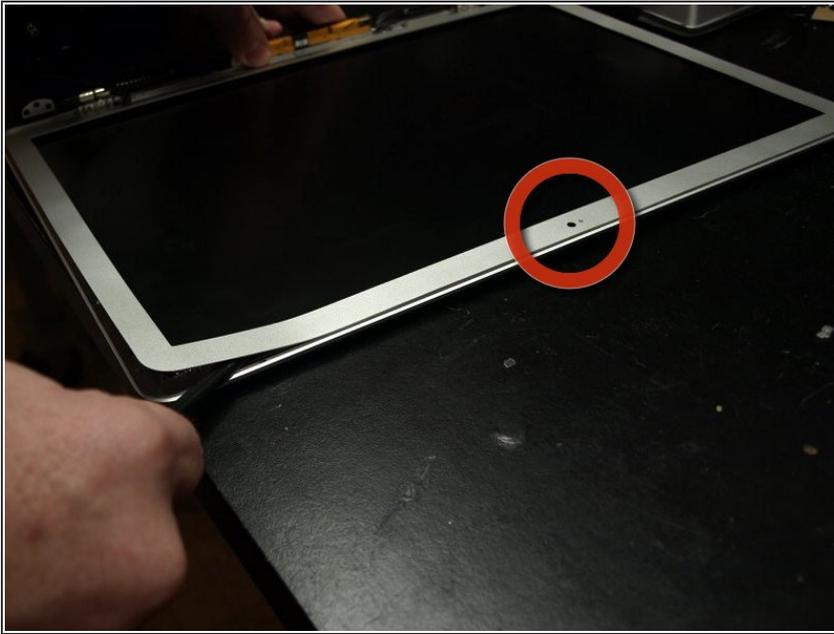
**⚠** Avoid placing the spudger within 20mm (3/4") of the built in camera. There is no adhesive in this location, and the spudger could damage the camera.
