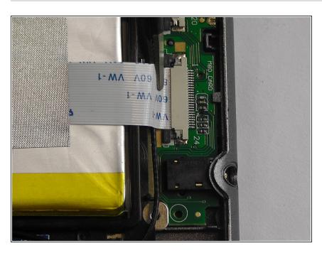
Re-insert the wire into the socket.
