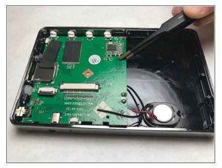
To remove mother board gently pull away from the top of the device to make sure the earphone jack it our of the slot.
