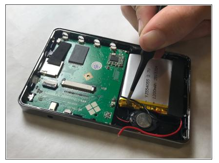
Now, carefully we will remove the battery. Find the leads, or the red and black wires going to the battery from the motherboard. To free the wires you must cut the wire near the battery leads. Make sure both ends are clean and have enough exposed wire.
