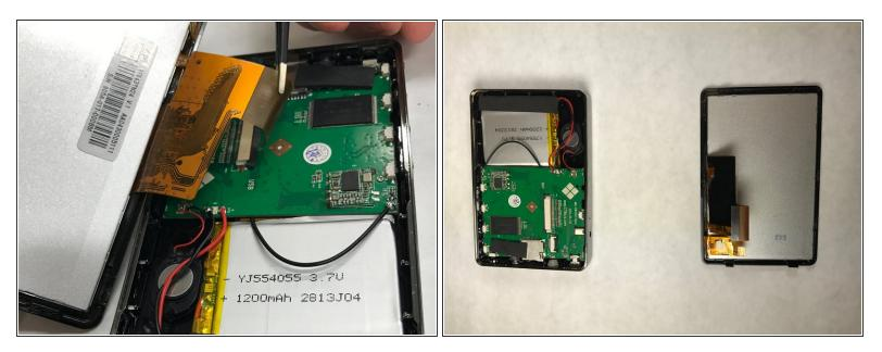
Using the prying tool, slide the black clip out. Pull the ZIF connector out and to the left, the screen is now detached from the motherboard.
