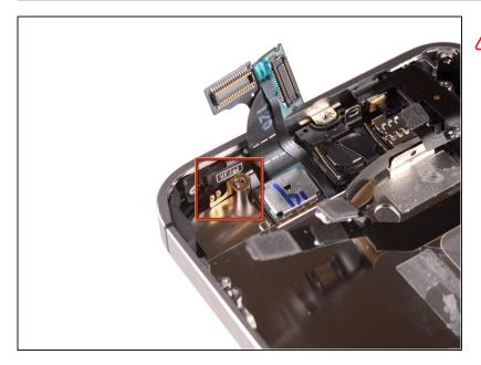
A Be sure not to lose the small grounding finger for the rear facing camera near the power button. This finger rests on top of the PCB, screwed down, and covered with the adhesive black plastic tape.
