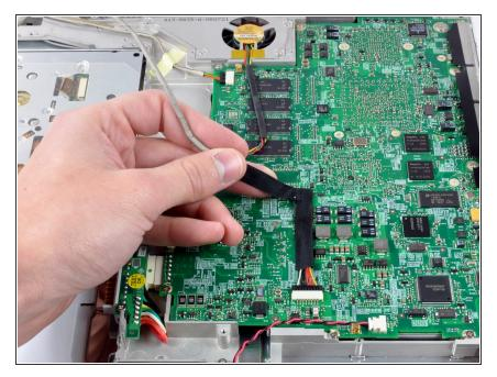
• Lift the DC-In cable from the adhesive attaching it to the logic board.
