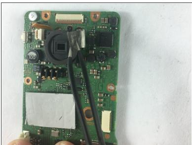
Using the precision tweezers, lift silver heat sync tape from motherboard.
