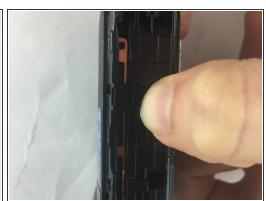
• Lift the two plastic tabs on the left side of the LCD screen and the single one on the right side on the black casing to open the device.
