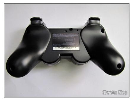
It is a little hard to put back on, but not impossible. You need to put it on over the R2, and L2 triggers, then you should push down on the back plate till' is snaps into place.
