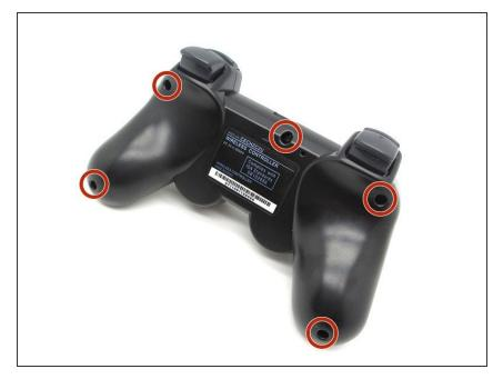
The screws are located in the holes of the in the back of the controller.
