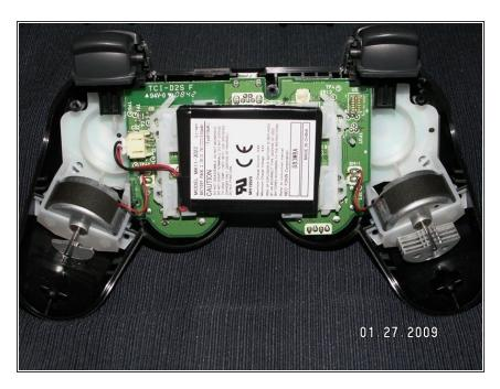
Lift up the battery, and move it away from the motherboard(the green board). Next you need to grab your pliers, and grip onto the piece of plastic that the wires lead to, be sure not to grab the socket that holds this plastic piece, and don't grab the wires. Once you have it you should slowly wiggle the plastic piece out of the socket.
