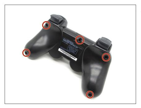
Once the 5 Screws are tightly screwed in you are done with the replacement of the battery.
