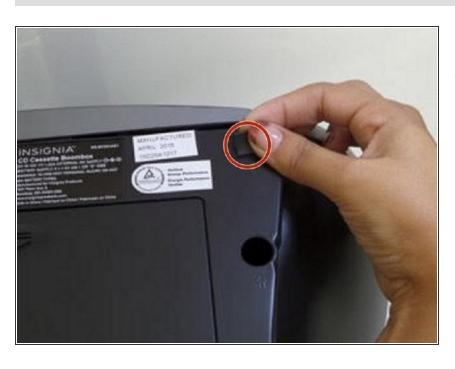
Peel off the two black square foams in front of the battery compartment to reveal a screw under each one.
