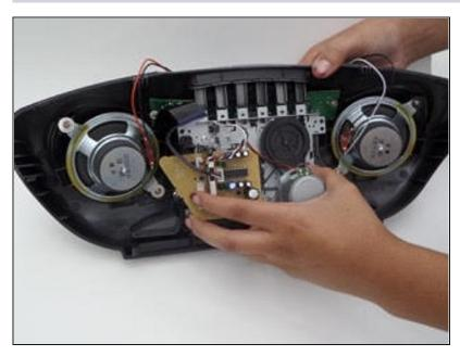
After disconnecting all the wires, the front panel is now free and easy to work on.
