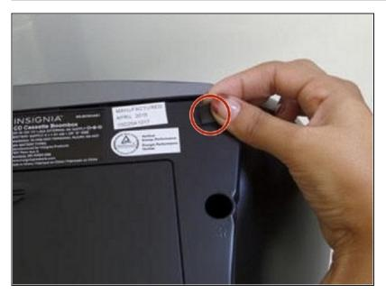
Peel off the two black square foams in front of the battery compartment to reveal a screw under each one.
