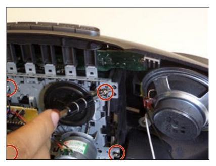
To remove the cassette unit, use a <u>2.5mm flathead</u> on the 4 screws holding the unit together.
