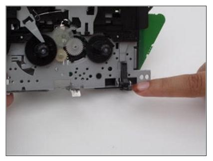
The door latch is located on the bottom corner of the cassette unit.
