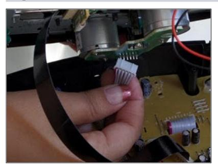
Unplug the red and pink wires connecting the top of the device to the motherboard
