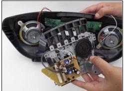
• While pressing the eject bottom, pull the cassette unit down and away from the front panel.
