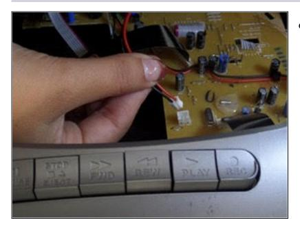
Start by unplugging the red and black cable connected to the motherboard
