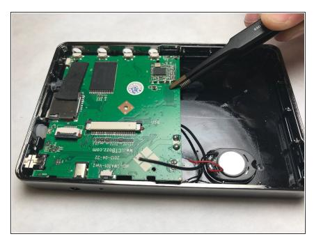
To remove mother board gently pull away from the top of the device to make sure the earphone jack it our of the slot.
