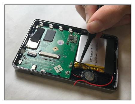
Now, carefully we will remove the battery. Find the leads, or the red and black wires going to the battery from the motherboard. To free the wires you must cut the wire near the battery leads. Make sure both ends are clean and have enough exposed wire.
