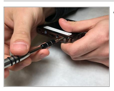
Remove both 4mm PH001 screws from the side panel.
