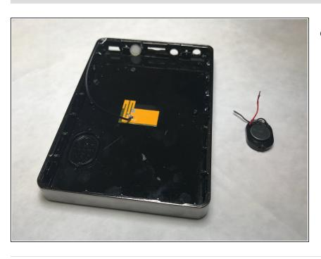
Use plastic spudger (prying tool) to remove speaker from casing mold.
