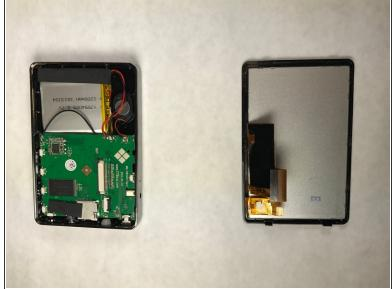
Using the prying tool, slide the black clip out. Pull the ZIF connector out and to the left, the screen is now detached from the motherboard.
