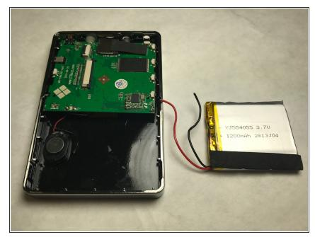
You will have to clean the connections and solder the new battery back into place. Just as before, you want to reconnect the new battery to the motherboard.
