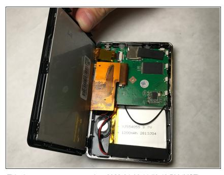
Gently turn screen over, to the side, to reveal the ZIF connector attached to the motherboard.
