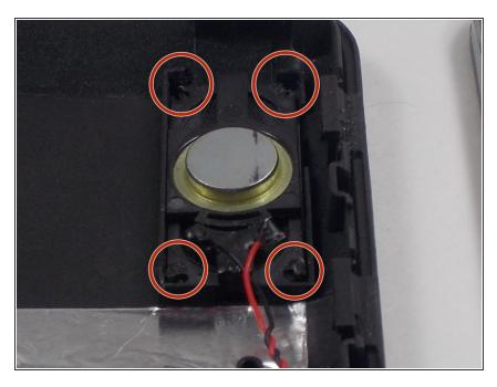
Desolder the soldering points that connect the speaker to the motherboard.
