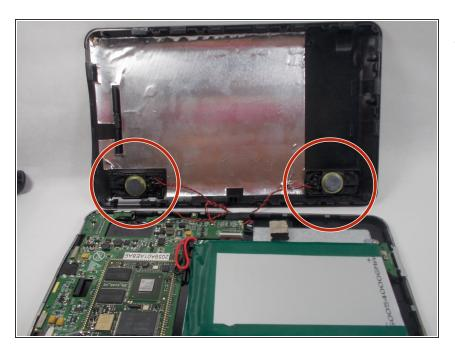
Once inside the device, locate the speakers on the inside of the back panel.
