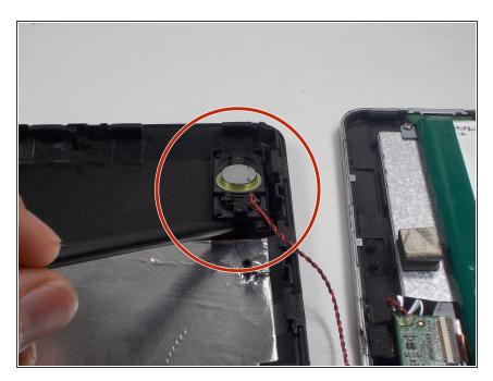
Use spudger to pry one speaker up off of the back panel.
