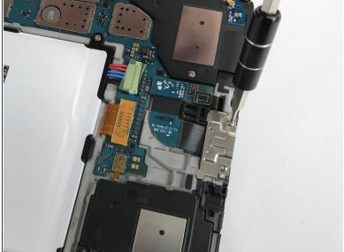
Remove the two 2.5mm Phillips #000 screws.
