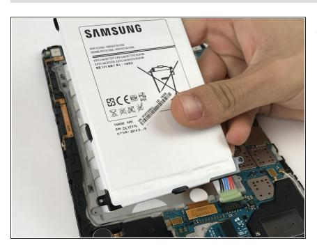
The battery should be completely disconnected and the new one can be installed.
