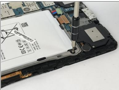
Remove the four 2.5mm Phillips #000 screws.
