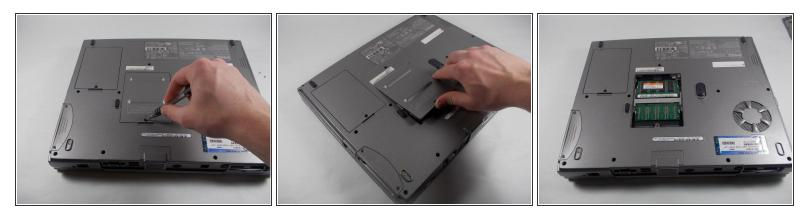
Remove the one Phillips #0 screw at the bottom-center of the panel covering the RAM and remove the panel.
